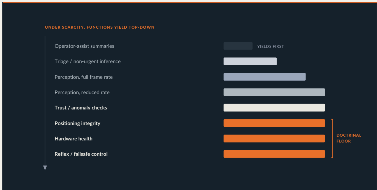
EXHIBIT 3 · WHAT YIELDS UNDER SCARCITY The airframe's shared budget forces a priority order. Advisory assistance and non-urgent inference shed first; perception degrades before safety, positioning, health, and deterministic failsafes. The degradation order is part of the system's operating doctrine.
